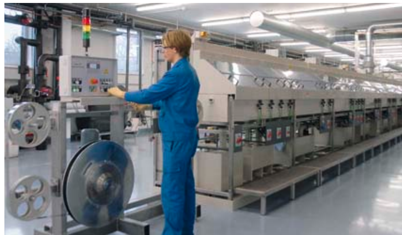
Pilot plant for the production of flexible copper-based CIS solar cells
