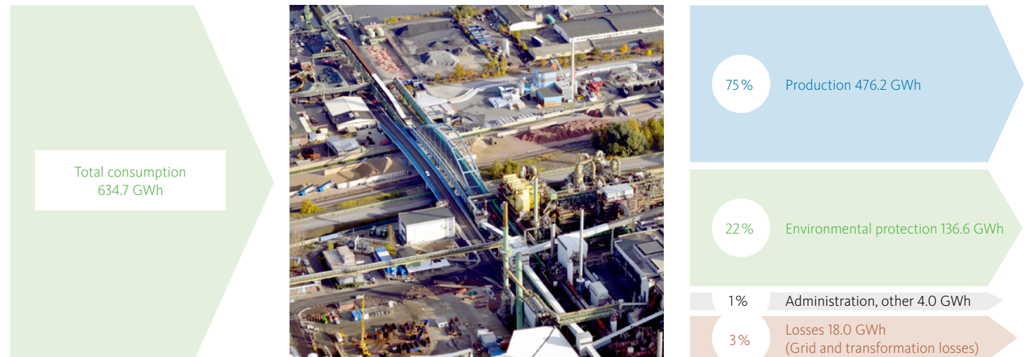
Fig. 2.15: Breakdown of energy consumption at the Hamburg site
