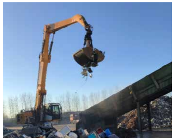
Releasing the electrical and electronic devices onto the feed conveyor of the MV-ZS facility
