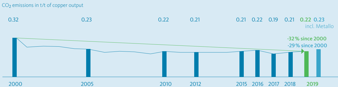
Fig. 1.8: CO 2 emissions from fuels in Aurubis Group copper production
