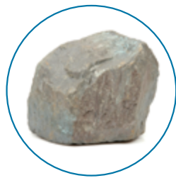
Iron silicate stone, with edges up to 450 mm in length, comparable to igneous rock
